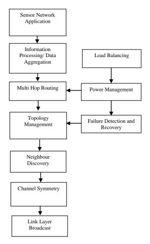
Fig. 2. Depends-on hierarchy for flat sensor network routing protocols. The function at the tail of an arrow depends on the function at the head of the arrow
