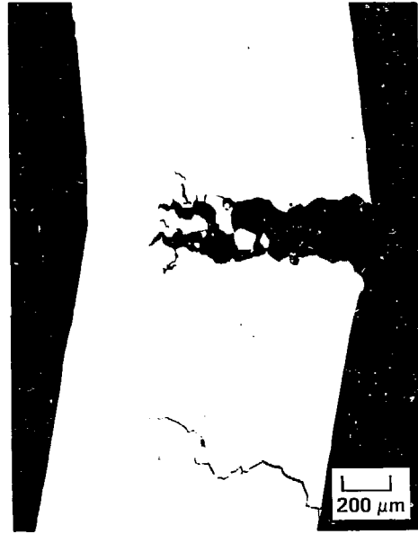
Fig. 5 Metallographic cross-sections of sensitized Type 304 U-Bend specimens showing IGSCC.
