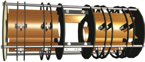
Fig. 4. Electrostatic quadrupole doublet with an integrated steerer as it will be used in the Frankfurt ion storage ring.
