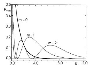
Fig. 1. The probability  $P_{mm}$  of a sudden process leaving the oscillator in its initial state *m* is plotted (for m = 0, 1, 2) versus the energy ratio  $\varepsilon \equiv \frac{E_C}{h_{rev}}$ .
