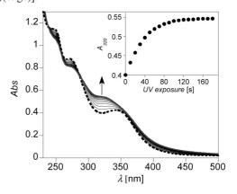
Figure 2. UV/Vis spectra of  $80 \ \mu\text{M}$  [Pt(cage)] in phosphate buffer at pH 7.4 photolyzed in 10 s intervals for a total of 180 s (initial spectrum at time zero is dashed line); inset: absorbance at 320 nm vs. irradiation time shows that the compound is completely photolyzed within 2 min.
