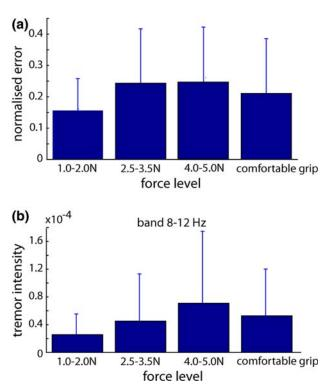
FIGURE 7. Effect of grip force on targeting error and tremor amplitude ( $\pm$ standard deviation). (a) Error vs. force at magnification ×10. (b) Illustrates the proportional power for 8–12 Hz bandwidth for different levels of grip force (1.0–2.0, 2.5–3.5, 4.0–5.0 N and subject's own comfortable grip).
