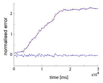
FIGURE 3. Effect of high-pass filtering on raw data. The original data is the jagged line, drifting away from zero. The smooth line laid over this is a low-pass filtered version of the data; note the tight fit of this curve with the original data. The jagged line along the *x*-axis is the high-pass filtered data; the very low frequency drift (<0.27 Hz) has been removed while retaining the higher frequency movement.
