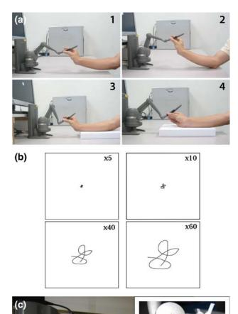
FIGURE 2. Experimental conditions. Four different postures were first examined (a), then magnifications up to  $\times$ 60 (b). The influence of grip force was also investigated using a force sensor attached to the PHANTOM stylus (c).
