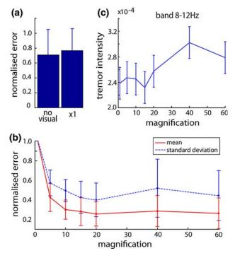
FIGURE 6. Mean position error (over the subjects) at various magnifications ( $\pm$ standard deviation). (a) Comparison of error in the 'blind' and  $\times 1$  magnification conditions. (b) Analysis of how the error depends on magnification. (c) Proportional power for 8–12 Hz bandwidth for increasing magnification ( $\times 1$ ,  $\times 20$ ,  $\times 40$ ,  $\times 60$ ).
