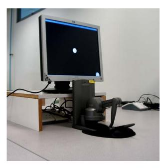
FIGURE 1. Experimental setup. The movement of the stylus measured by the PHANTOM desktop interface is displayed as a disc on the screen. The subjects must maintain this disc in a nominal position. In some trials the subject must additionally maintain the required grip force within a given range as measured by the force sensor.
