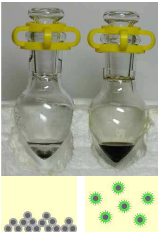
Fig. 5. Dispersion of the oleic acid-coated Fe 16 N 2 / metallic oxide nanocomposite in chloroform. The magnetic fluid ( right ) was composed of the oleic acid ( green )-coated iron nitride/ metallic oxide nanocomposite ( dark gray light gray ) dispersed in chloroform ( yellow ).
