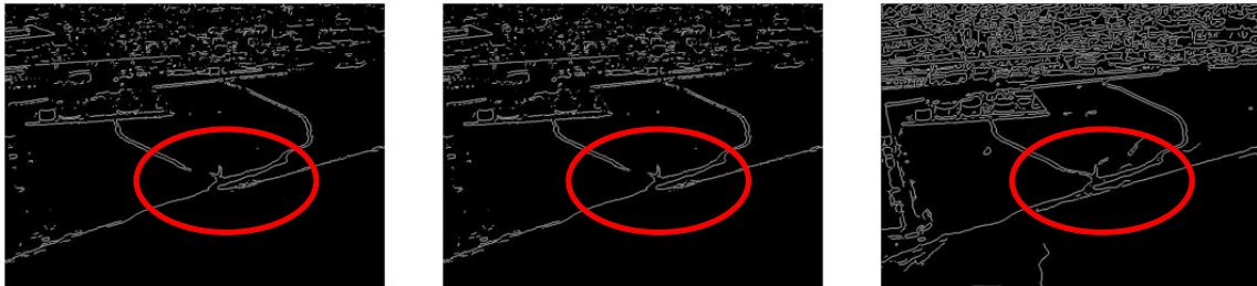
Fig. 11. Comparison of edge detection algorithms/filters: a) Prewitt; b) Sobel; c) Canny.
