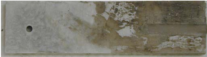
Figure 2 MORCOCOat SP-P after 100 hr. immersion in BL smelt. Showing minimal to no reaction.
