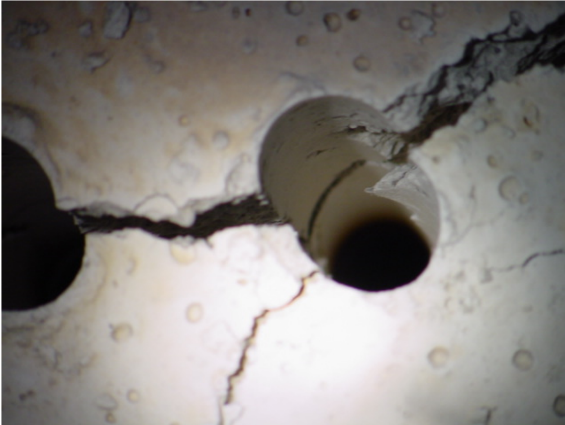
Figure 4 Enlargement showing critical delamination failure at 5-6" in depth and accompanying transverse cracking.
