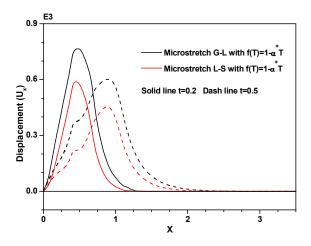
Figure 4: Displacement  $U_x$  distribution at z=0 versus x under different generalized thermoelastic theories.
