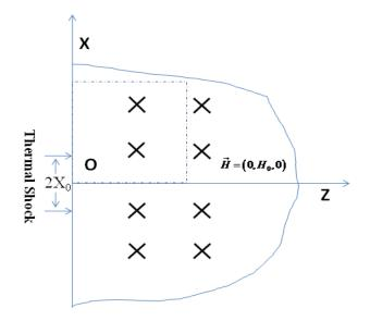
Figure 1: A half-space placed in a transverse magnetic field whose surface suffers thermal shock.
