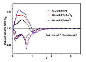
Figure 14: Induced electric field  $(E_z)$  distribution at z=0 versus x under different forms of temperature dependent material properties.
