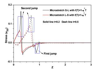
Figure 5: Stress ( $\sigma_{zz}$ ) distribution at x=0 versus z under different generalized thermoelastic theories.
