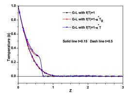
Figure 9: Temperature ( $\theta$ ) distribution at x=0 versus z under different forms of temperature dependent material properties.
