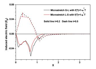
Figure 8: Induced electric field ( $E_z$ ) distribution at z=0 versus x under different generalized thermoelastic theories.
