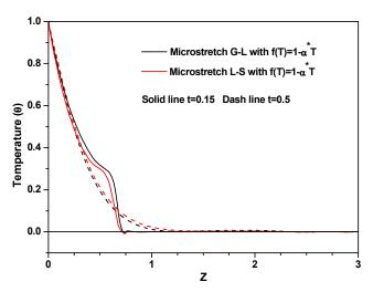
Figure 3: Temperature distribution at x=0 versus z under different generalized thermoelastic theories.
