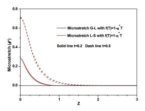
Figure 6: Microstretch ( $\phi^*$ ) distribution at x=0 versus z under different generalized thermoelastic theories.
