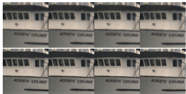
Fig. 13. Zoom-in of “Acoustic Explorer” sequence frame no. 25-28 (object is 2 miles from camera). Top: input video sequence with contrast enhanced by gray level grouping (GLG). Bottom: Processed video by applying the proposed method to the output of GLG.
