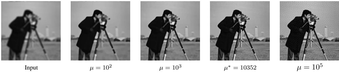
Fig. 1. TV/L2 Image recovery using different choices \mu . The optimal (in terms of PSNR compared to the reference) is \mu = 10352 . The image is blurred by a Gaussian blur kernel of size 9 \times 9 , \sigma = 5 . Addition Gaussian noise is added to the image so that the blurred signal to noise ratio (BSNR) is 40dB.
