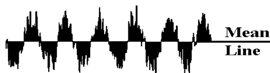
Figure 1. Mean line of a surface profile
