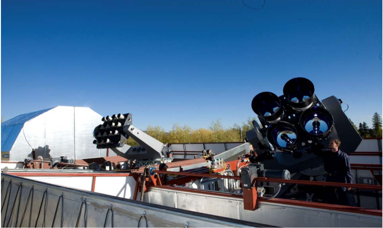
Figure 3. The RAPTOR-T multi-color follow-up telescope array (foreground) and the RAPTOR-K sky monitoring array. These fully autonomous robotic telescopes monitor the night sky for interesting targets and make real-time follow-up observations without “humans in the loop”.
