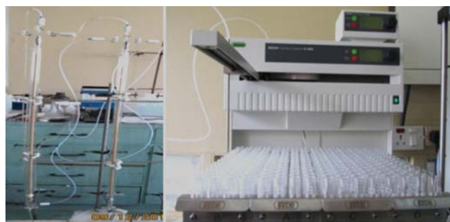
Fig.7: Experimental setup of chromatographic separation of Gd isotopes
