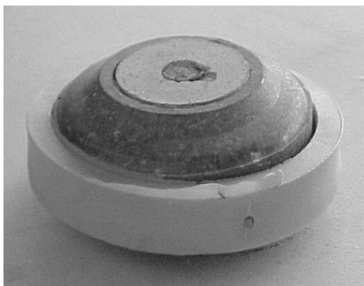
Fig. 3. Gasket with the PVC ring
