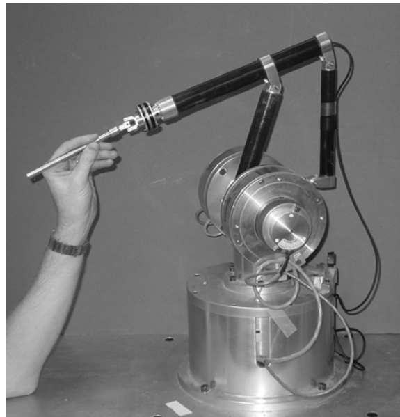
Fig. 4. Three degree-of-freedom master manipulator.
