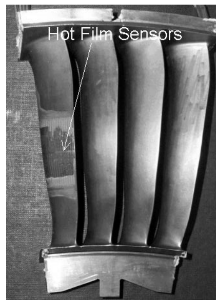
Figure 4 NGV2 of the BR715UHL LP turbine showing the hot film array of sensors on the right hand aerofoil.
