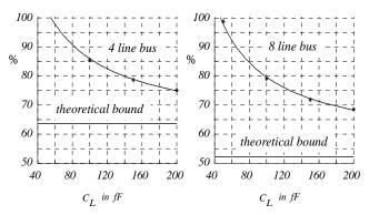
Figure 13: Normalized energy using CRT (HSPICE simulation)
