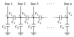
Figure 1: Sub-micron energy-equivalent Bus Model
