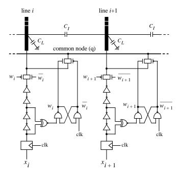
Figure 10: Efficient CRT - Driver
