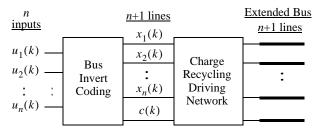
Figure 8: Combination of CRT with Bus Invert coding
