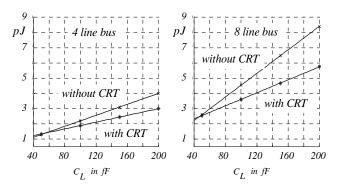
Figure 12: Average energy per cycle of a 4 and 8 line buses with and without CRT
