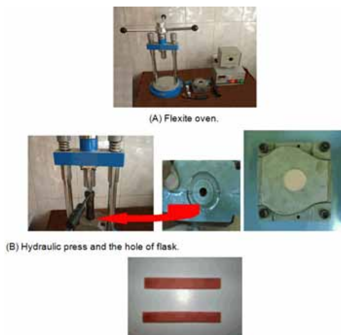
Figure 2: Flexite Samples prepared by machine injection type (ZB-A) oven. (A) Flexite oven, (B) Hydraulic press and the hole of flask, (C) Flexite (Valplast) samples.
