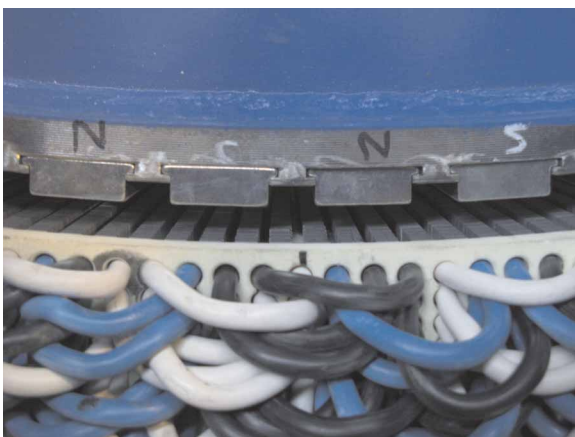
Fig. 5 A photograph showing the air gap, PM, and cable windings
