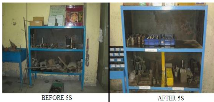
Figure 3: There are 5 tool boxes like shown above, tools were placed haphazardly manner but after 5S everything was placed after its name and name slips were put for every tool.
