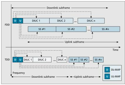
■ Figure 1. Frame structure with FDD and TDD.
