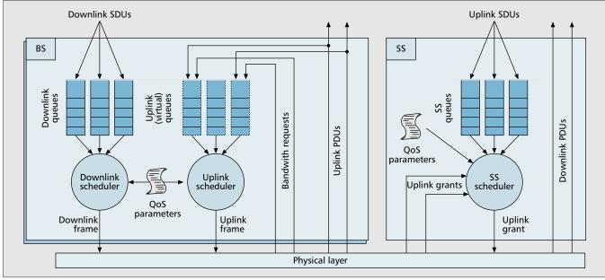
Figure 2. QoS functions within the BS and SSs.
