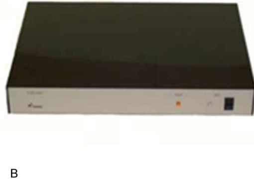
Figure 2. Photograph of the miniature recording telemetric system. This system consists of two separate parts, (A) telemetric implant unit, which can be used inside or outside of the animal body to transmit signal, and (B) wireless receiver, which can amplify and convert the signal.
