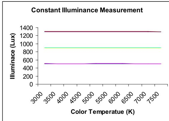
**Figure 3 :** Measuring LED color temperature while maintaining illuminance values constant
