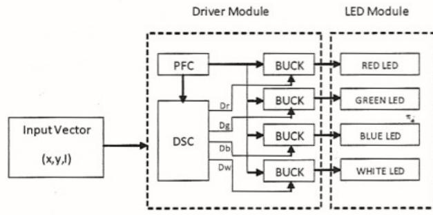
**Figure 2 :** Schematic of RGBW LED source
