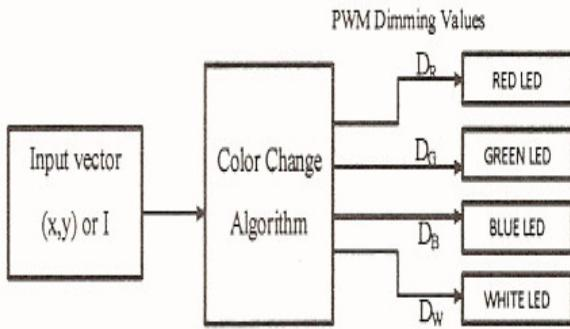
**Figure 1 :** Block diagram of RGBW LED color change algorithm
