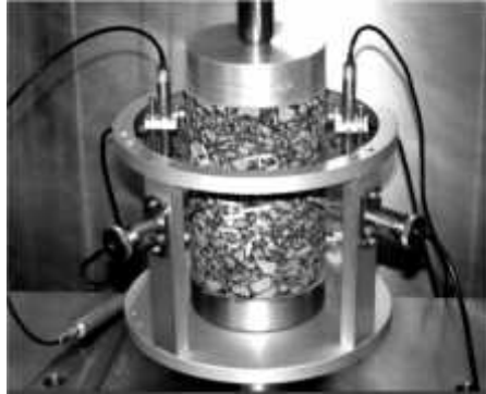
Figure 5. Flow Number Test Setup, Unconfined Condition
