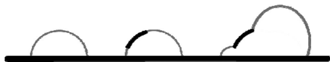
Figure 13. Sodium could block dendrite growth by depositing on electrochemically active lithium faces. Foreign surface effects of lithium and sodium could prevent further deposit in that area while the rest of the nuclei continues to grow resulting in a dimple.
