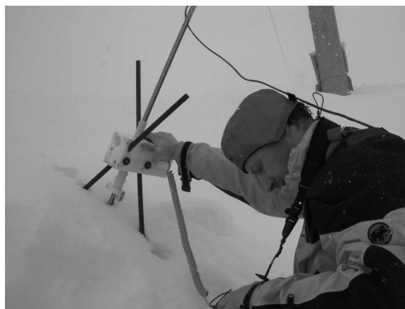
Figure 1: SMP profiling parallel to the manual snow profile and the stability test (Photo: SLF/A. Raez).
