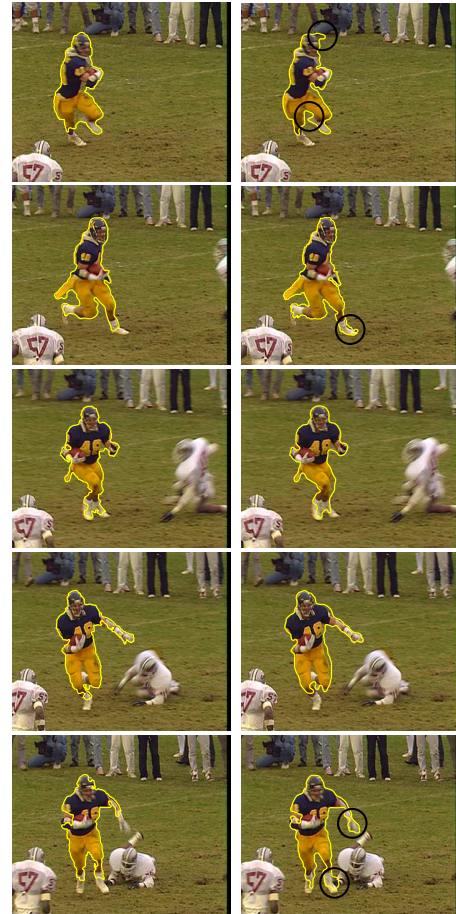
Figure 10: Tracking on sequence ‘Football’: comparison between global motion approach (first column) and local motion approach (second column) on frames 73, 77, 81, 85, and 89. The segmentation is more accurate with the local motion approach (the main differences are highlighted by circles).
