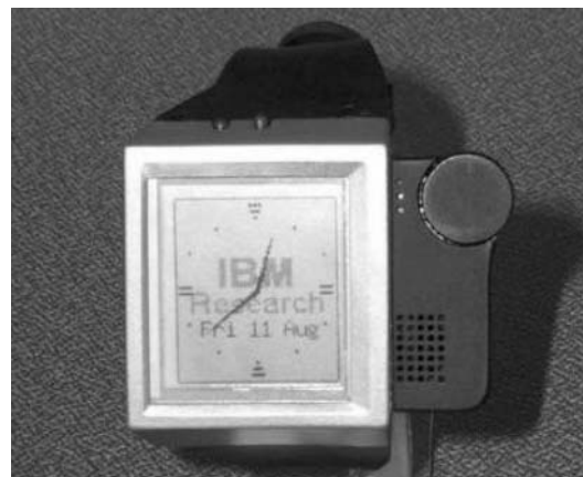
Fig. 1. Wrist watch computer with low resolution liquid crystal display.
