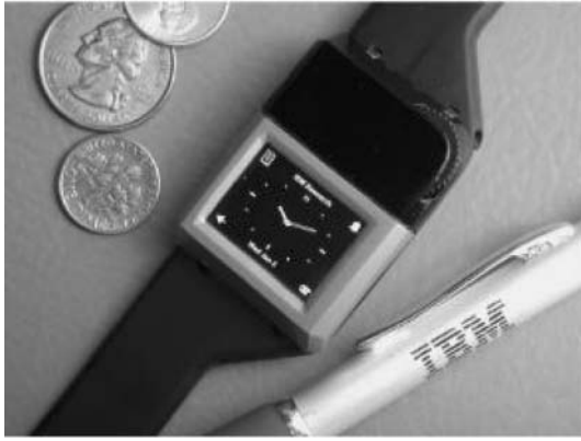
Fig. 2. Wrist watch computer with high resolution organic light emitting diode display.
