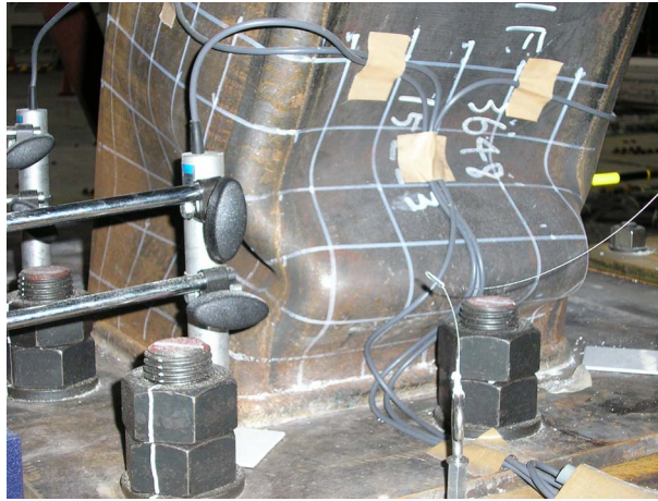
Figure 8. Severe local buckling of HSS column at baseplate, with drift ratio of 0.19 (from View B depicted in Figure 6).
