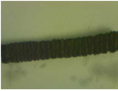
Fig. 5. Fabricated platinum fiber-reinforced PPy tube.
