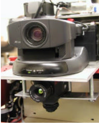
Figure 1: Thermal camera mounted on robot
