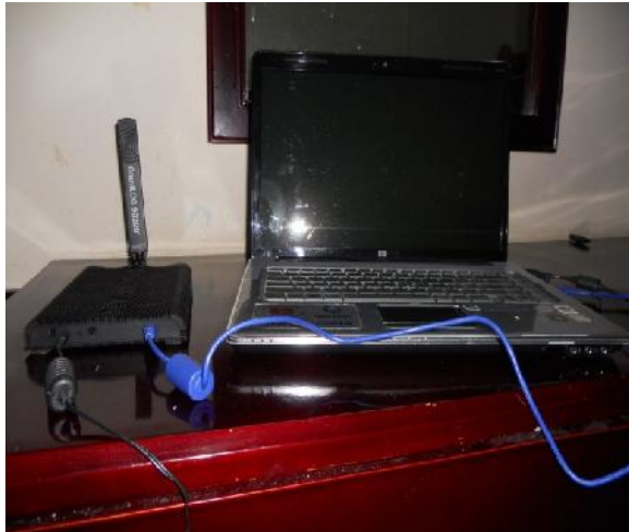
Fig. 1. Setup used for Spectrum Occupancy measurement
