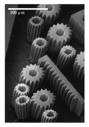
Fig. 2. SEM micrograph of cogs produced in bulk PMMA using a direct-write 2 MeV proton beam.
