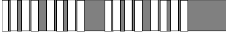
Fig. 1. A schematic segment of a period of the 16th order one-dimensional block-hierarchical model of masses (light color rectangles) and partings (dark color rectangles)
