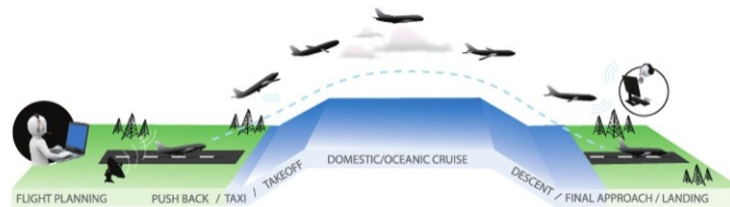
Figure 1. Flight phases cycle.
