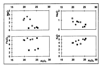
Figure 4. Chemistry of soil and rock samples, from this study and from Warr & Rice (1993). Filled symbols indicate non-chloritic samples, open symbols indicate chloritic samples. Square symbols indicate soil samples, diamond symbols indicate rock samples.
