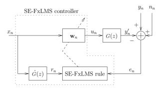
Figure 1: Block diagram of the signed-error FxLMS algorithm
