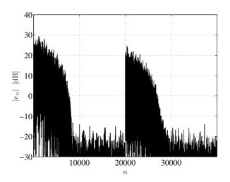
Figure 6: Convergence of the SE-FxLMS.  $g_n$ : acoustic system.  $\mu = 2 \cdot 10^{-2}$ , N = 10,  $\varepsilon = 0$ . MAE<sub>ss</sub> is 0.0225 and 0.0219 in the first and second steady-state interval, respectively,  $\bar{E}_{ss}^{a} = 0.391$ .
