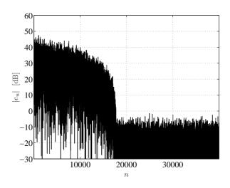
Figure 3: Convergence of the SE-FxLMS with simple delayed feedback:  $G(z) = z^{-50}$ .
