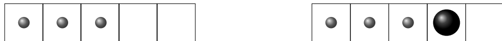
FIGURE 4.2: A task stack before and after spawn operation. The big ball shows a new spawned task.
