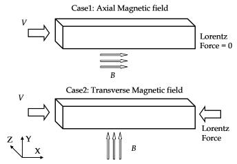
Fig. 1. Schematic showing the direction of Lorentz Force
