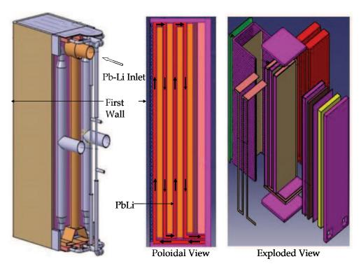
Fig. 21. Details of LLCB- TBM, Wong et al. (2008)
