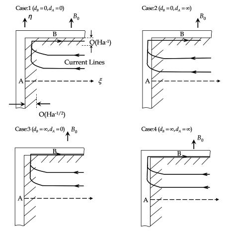
Fig. 9. Schematic of the current lines in the rectangular duct
