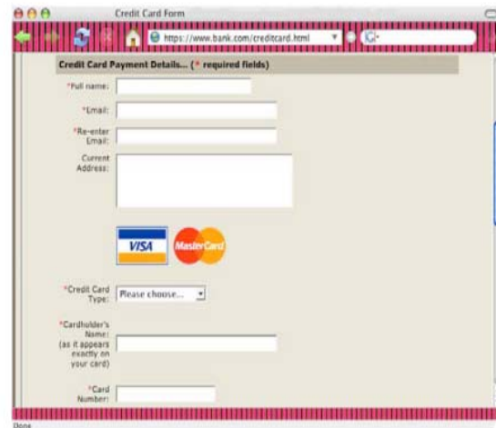
Figure 5: The browser displays the visual hash as a border around the authenticated website
