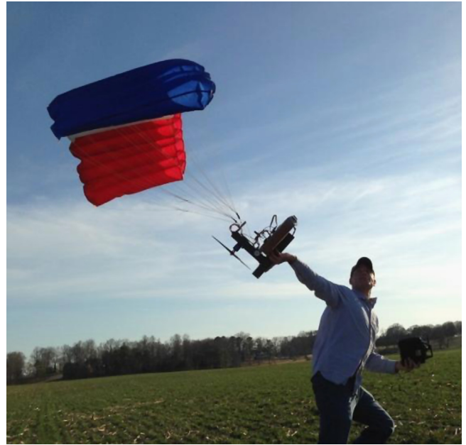
Fig. 7. Photo of experimental parafoil-payload system with embedded GPU (located in brown box on payload).
