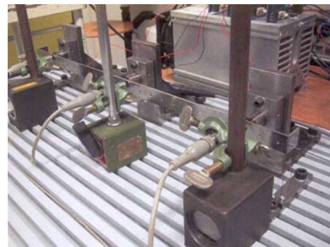
Figure 5. Flexible beam with three actuators.
