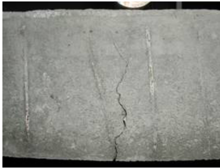
a) Crack appeared near the mid-span of specimen
