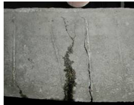
b) The adhesive flowed out from the broken-open fibers, filled /repaired the crack
