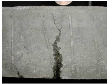
b) The adhesive flowed out from the broken-open fibers, filled /repaired the crack
