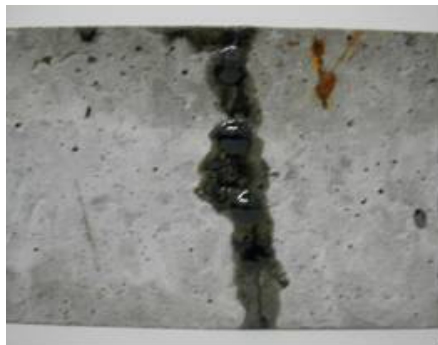
a) Crack appeared near the mid-span of specimen
