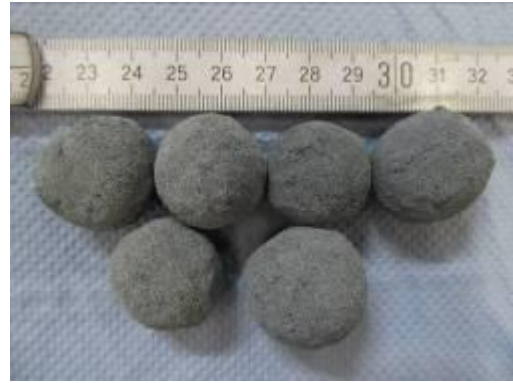
Figure 5: Alumina wood-charcoal pellets used in experiments.
