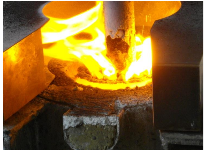
Figure 6: Furnace operation and Melt Sampling
