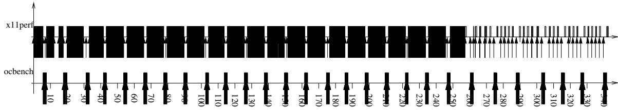
Figure 7. trace of an ocbench scheduled by a hard CBS, with overloaded X server.
