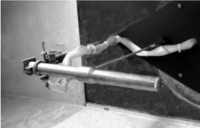
Fig. 4 Probe mounted in a low-speed wind tunnel
