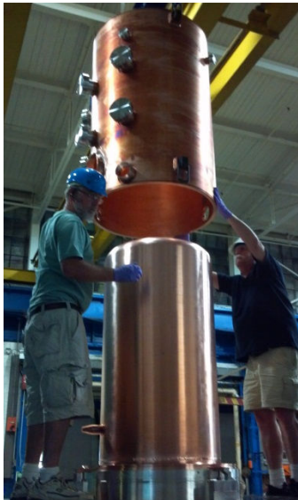
Figure 2: Positioning of outer conductor before electron beam welding.
