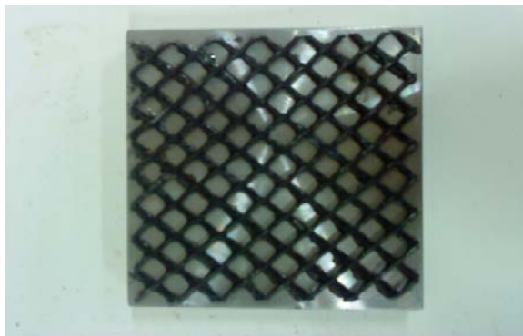
Fig. 4 Rough base of square footing.
