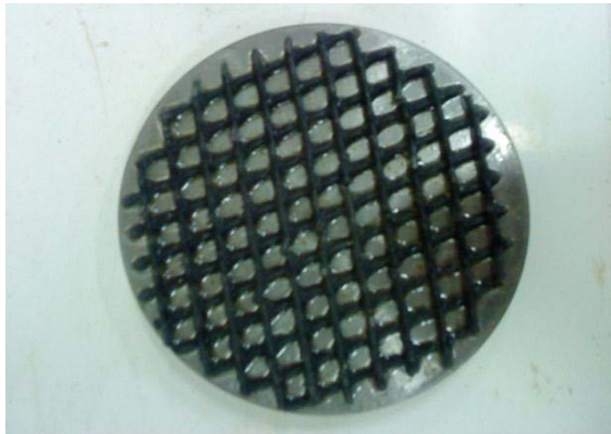
Fig. 3 Rough base of Circular footing.
