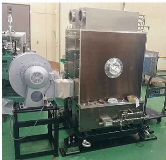
Figure 1: Shroud of the second harmonic cavity. The cavity is a single cell type using forced air cooling.
