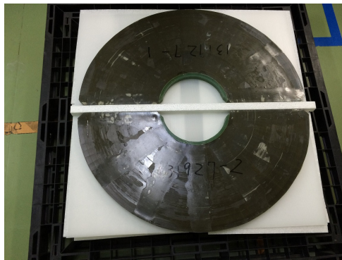
Figure 3: A cut core for the air cooled cavity.
