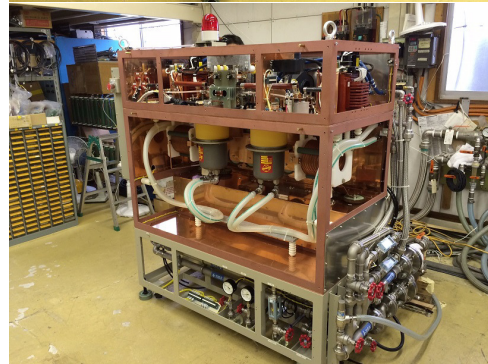
Figure 6: Tube amplifier for the second harmonic RF.
